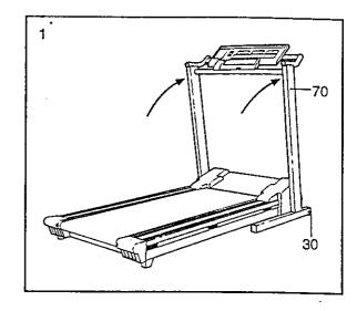
2. Remove the four Handrail Screws (103) from the posts on the left and right Uprights (70). Slide the upper end of a Handrail (101) onto the post on the left Upright. Note: It will be necessary to pivot the Handrail to the side and back repeatedly (see arrow A) while pushing on the Handrail to slide it fully onto the post. Next, pivot the lower end of the Handrail down and pull back on it (see arrow B) to align it with the hole in the left Upright.
